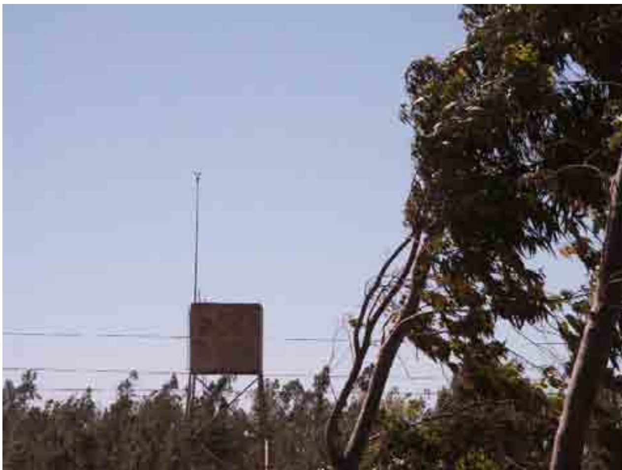
Figure 6-6: RTPC Anemometer with Surrounding Vegetation (Wind Breaks)
