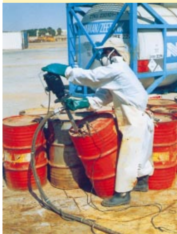
Transfer of dieldrin from drums into an Isotank in Mauritania.
