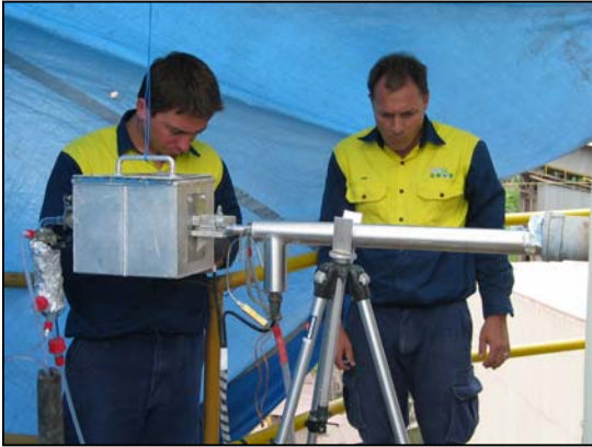
Installation of the tempered probe in one of the four sampling points
