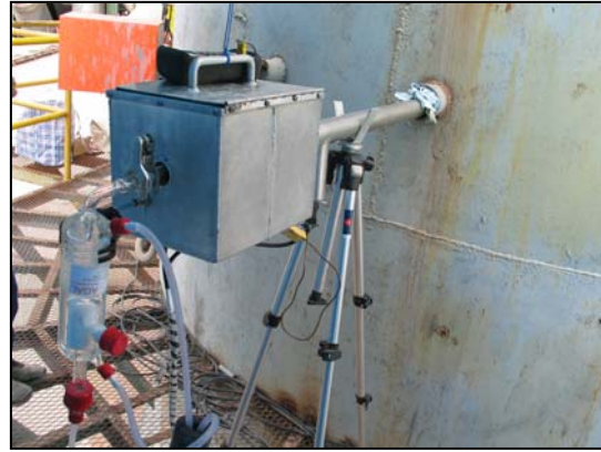
Installation of the tempered probe in one of the four sampling points
